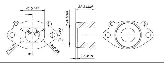
EXHAUST FITTING WITH Ø24 RESTRICTOR MARKING
